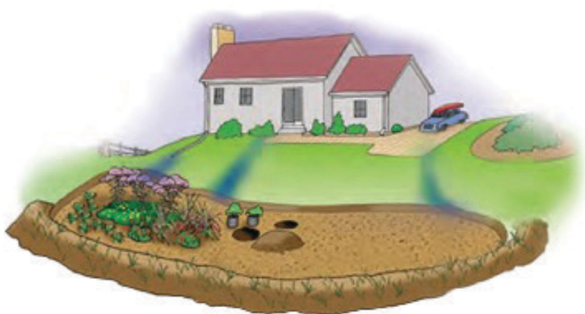
FIGURE 6. A berm is critical to help hold the water inside the rain garden.
