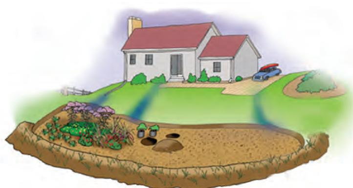
**FIGURE 6.** A berm is critical to help hold the water inside the rain garden.
